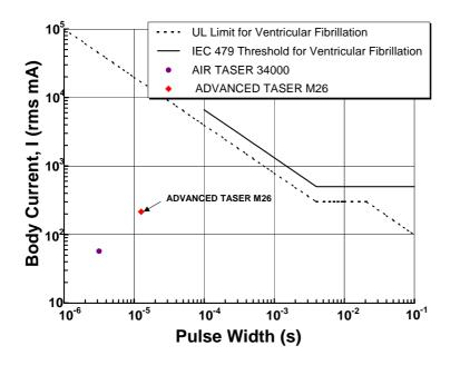
**Figure 1** – Taser graph packaged with Taser marketing material delineating unreproducible curves and invalid claims for the Taser M26 when compared to UL and IEC standards.
